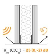
plasterboard panels with FIRE SEALING SILICONE to restore the sound reduction index
